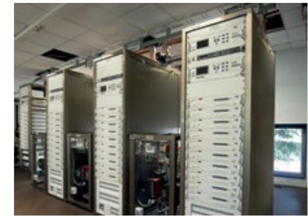
Suministro de la serie TLWH7900 de transmisores de TV eficientes de alta potencia. Supply of the TLWH7900 series of high-efficiency high-power TV transmitters.
