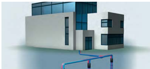
FIGURE 2-6 VERTICAL BOREHOLE HEAT EXCHANGER 7 (BHX) SYSTEM
