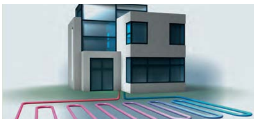
FIGURE 2-5 HORIZONTAL GROUND HEAT EXCHANGER SYSTEM 6
