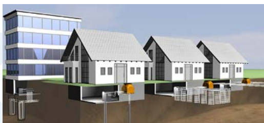
FIGURE 2-7 FOUNDATION HEAT EXCHANGER (FHX) SYSTEM USING ENERGY PILES 8
