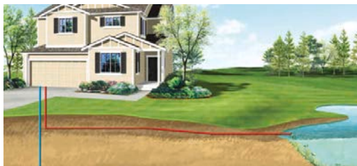
FIGURE 2-3 OPEN LOOP GEOTHERMAL CIRCUIT
