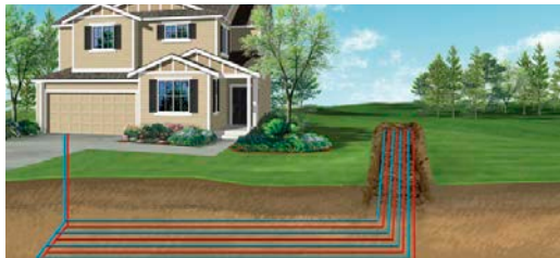
FIGURE 2-4 CLOSED LOOP GEOTHERMAL CIRCUITS
