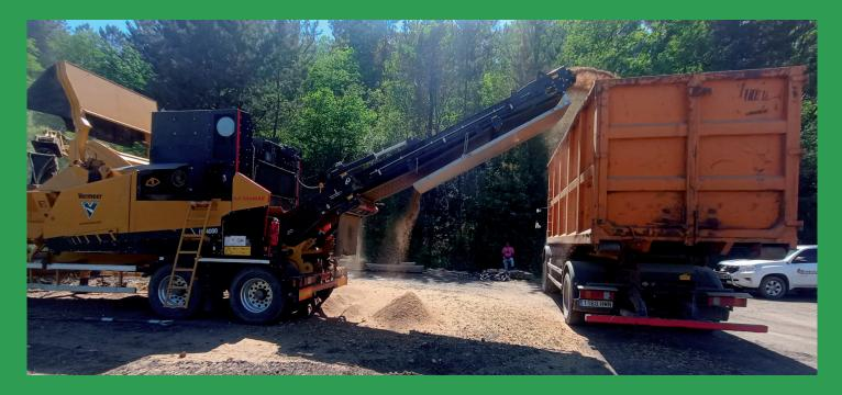
Bioenvironmental improvement of topsoil to be used for site restoration by incorporating shredded tree material from felled trees
